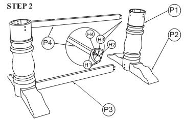
Assemble leg prongs P2 to both Pedestal Legs P1, then align Bottom Stretcher P3 and Top Rail P4 to connect both Pedestal Legs.
